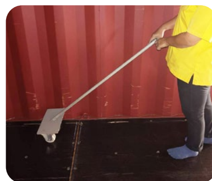
Magnetic tool used to remove metallic foreign objects
