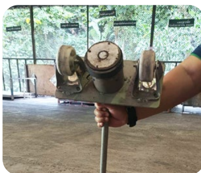
Metal detector used to detect metallic object contamination
