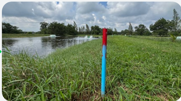
✅ Steel stakes are clearly marked with visual indicators
