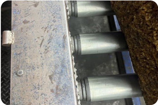
❗ The chain guard was too short, exposing the roller conveyor chain.
