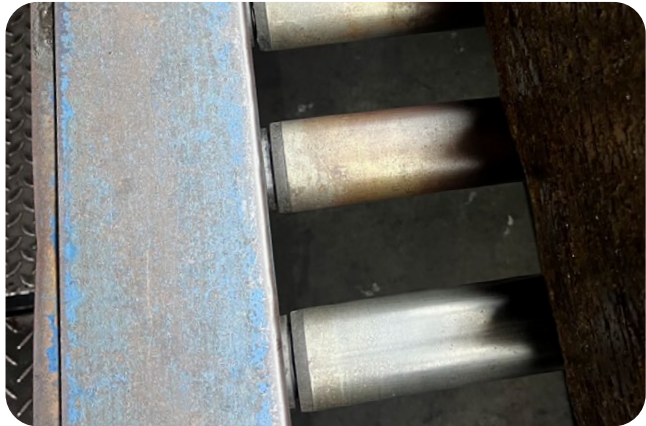
✅ A complete chain guard was installed, covering the conveyor chain and reducing the risk of entanglement.
