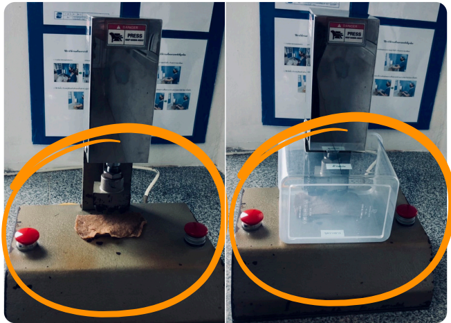
Before: Without safeguard & with temporary safeguard
