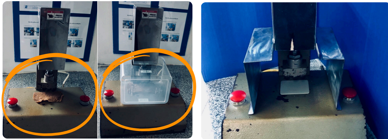
Before: Without safeguard & with temporary safeguard
