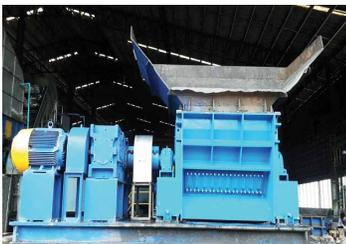
BJ4 redesigned our cutter machine efficiency by using same motor of 90Kw. Therefore, it enabled us to increase production efficiency by 25%.
