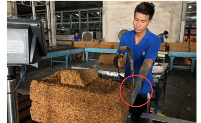
▲ Stainless steel gloves are worn to prevent injuries when using a coping saw to cut the rubber at our Standard Thai Rubber (STR) production plants
